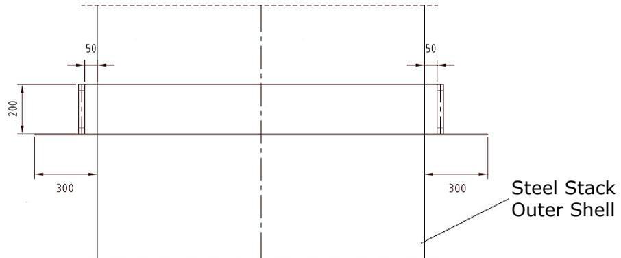
**Roof Flange for Roof with Slope**
